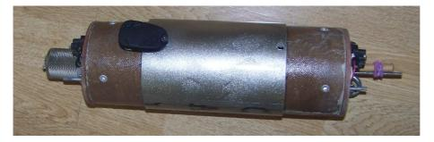
In my rockets what I do is use screw switches to turn on my altimeter so the hole for the screw switch is also used for exchanging pressures.
